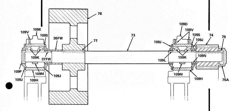
Roller Bearings are lubricated when press is shipped and will require additional grease approximately every three months. One shot or one stroke of grease gun is sufficient.
